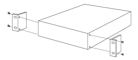
Figure 2-1: Mounting Bracket Orientation
